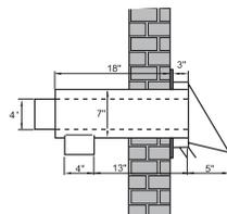
FT-4 Concentric Pipe-in-Pipe Termination
