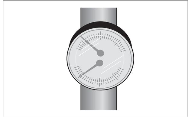
Fig. 26 Pressure and temperature gauge
