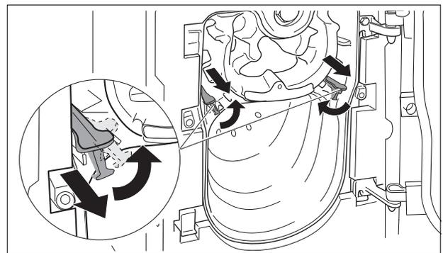
Fig.43 Adjusting the flue baffles
