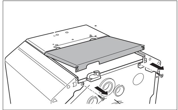
Fig. 28 Top rear cover removal
