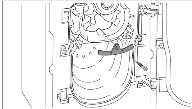
Fig.46 Removal of flue blocking plate
