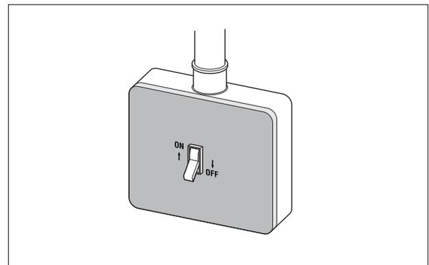
Fig. 49 Heating system shut down (with aquastat)
