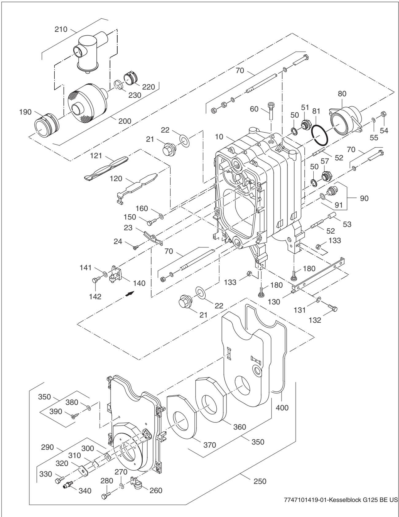
Fig. 60 Boiler block and burner door
