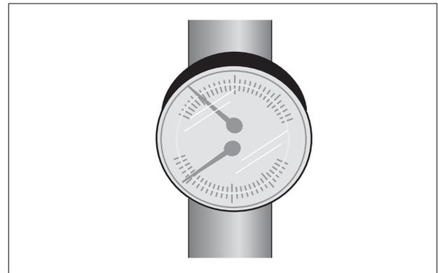
Fig.38 Pressure and temperature gauge
