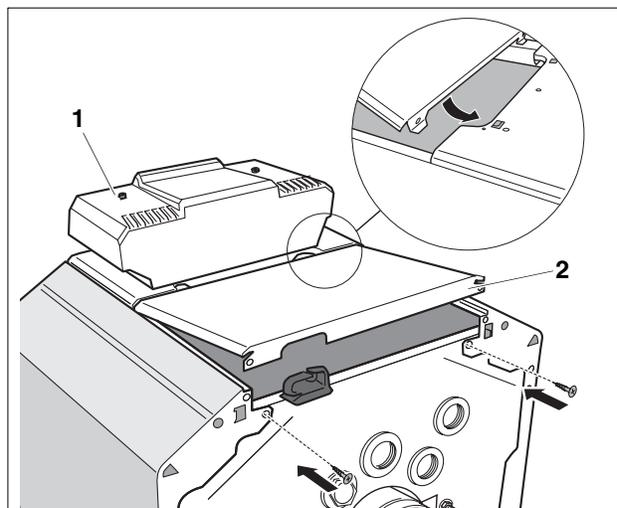
Fig. 37 Installation of rear top cover
