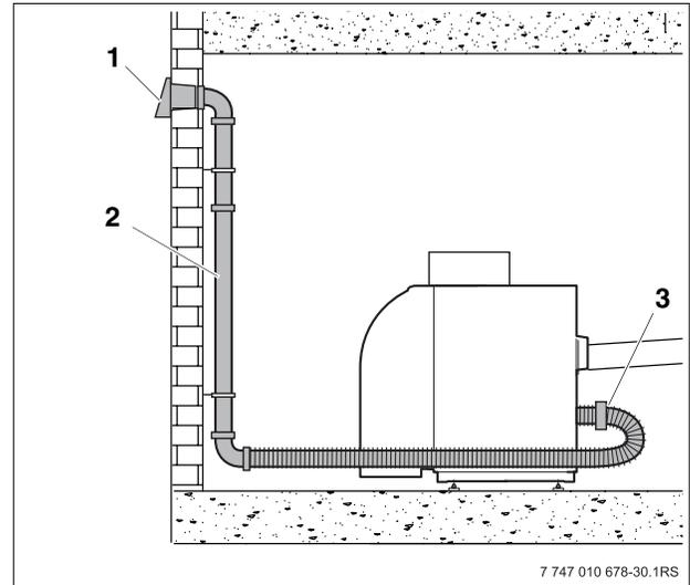
Fig. 20 Combustion air supply system
