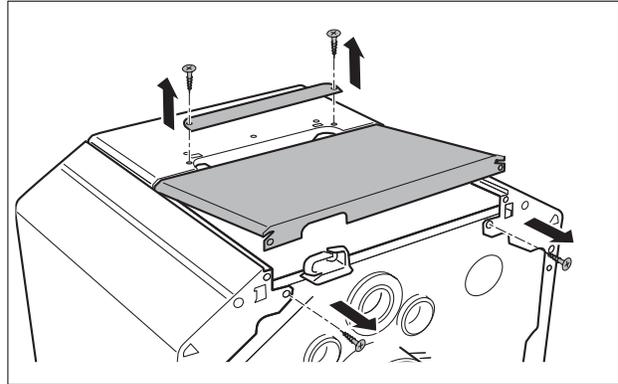
Fig. 30 Removal of rear top cover and top cover plate
