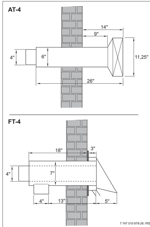
Fig. 15 Aerocowl (AT-4) and Concentric (FT-4) termination
