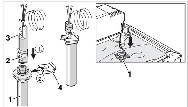
Fig. 35 Routing and connecting of capillary, sensor and electrical wiring
