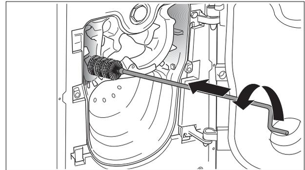
Fig. 51 Brushing out of flue passages
