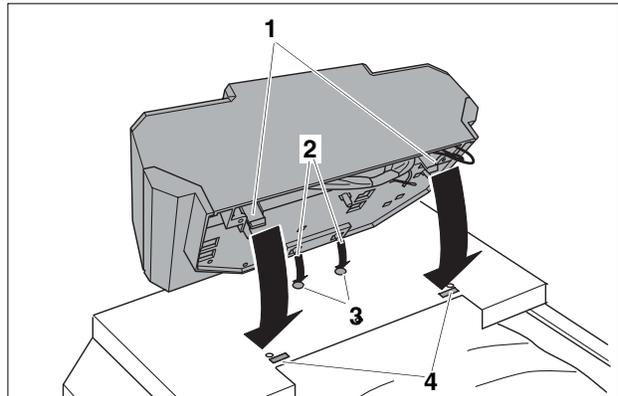
Fig. 31 Installation of control
