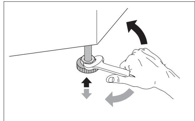
Fig. 11 Leveling the boiler
