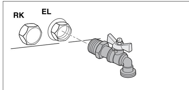
Fig. 24 Boiler Drain installation
