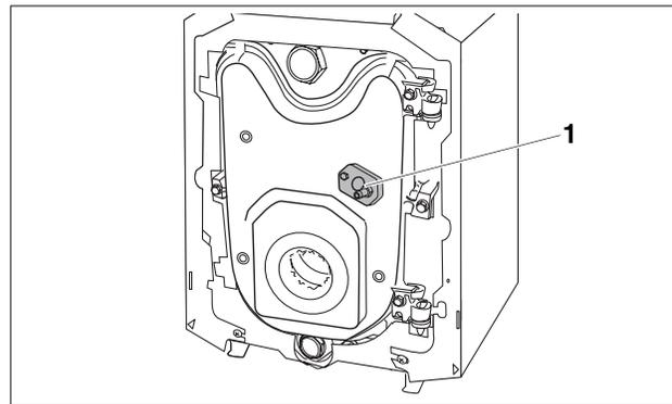
Fig.42 Pressure test port on burner door
