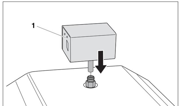
Fig. 29 Installation of Honeywell aquastat
