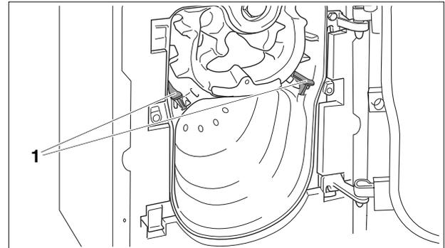
Fig. 50 Opening of burner door
