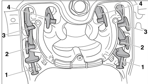
Fig.45 Blue baffle plates for fresh air operation
