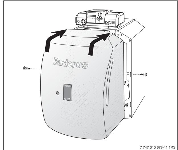
Fig.47 Installation of burner cover
