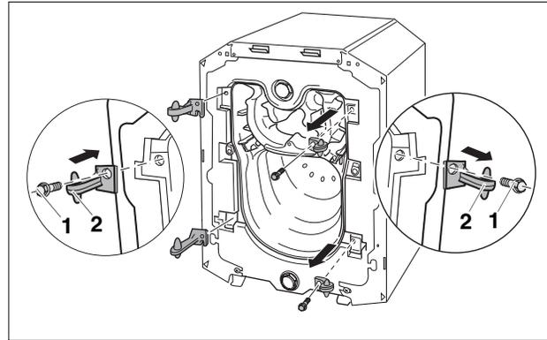
Fig. 8 Reversing burner door (boiler block)
