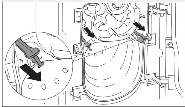
Fig.44 Removal of the flue baffles
