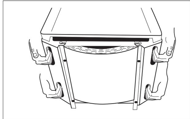
Fig. 5 Lifting and carrying the boiler
