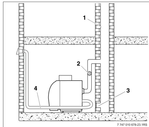
Fig. 12 Masonry chimney installation
