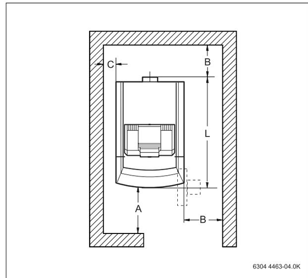
Fig. 7 Clearance dimensions for G125 boilers
