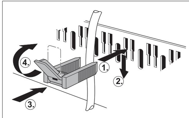
Fig. 36 Secure wiring with cable clips
