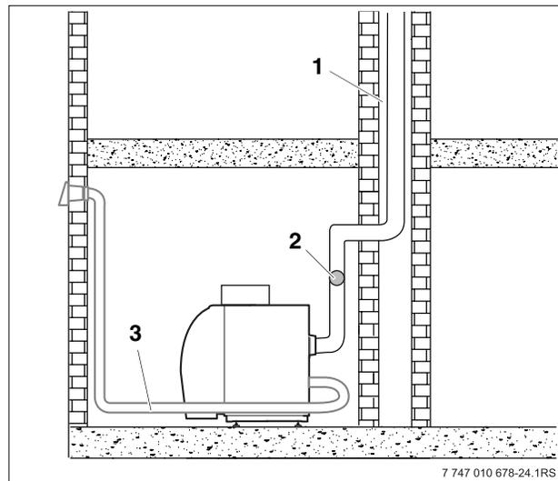
Fig. 13 5" Chimney liner installation
