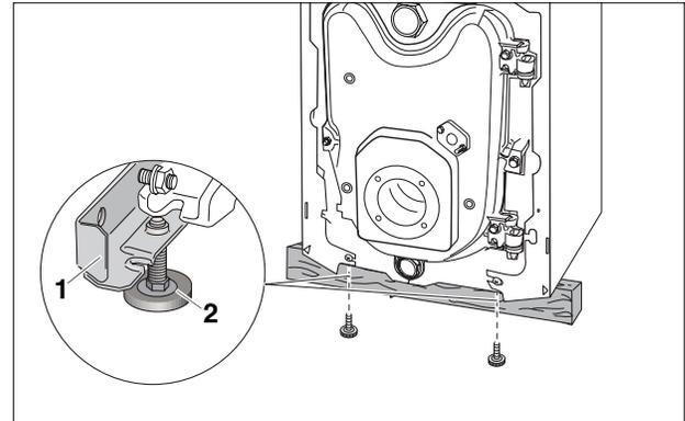
Fig. 10 Installation of boiler feet
