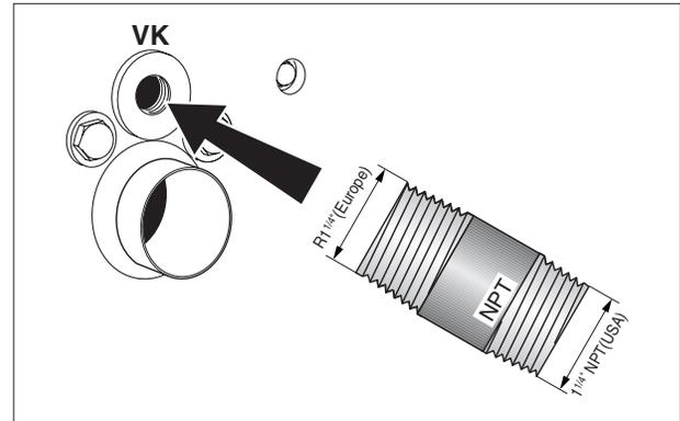
Fig. 22 Measuring thread length on 1-1/4" conversion nipple
