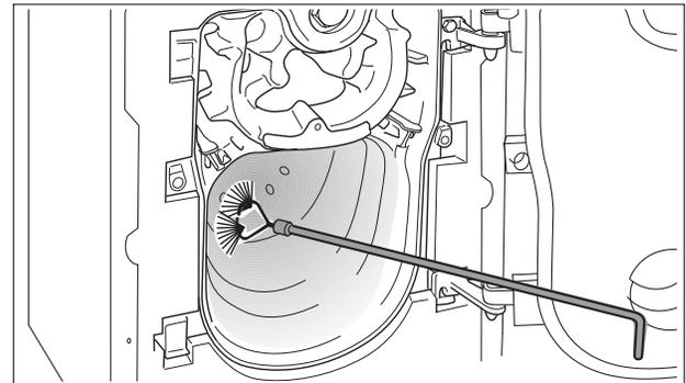
Fig. 52 Brushing out the combustion chamber
