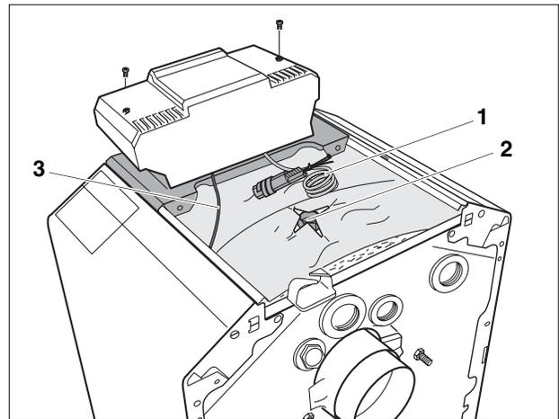
Fig. 34 Routing and connecting of capillary, sensor and electrical wiring
