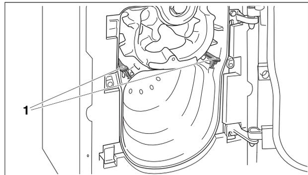
Fig.39 Opening the burner door
